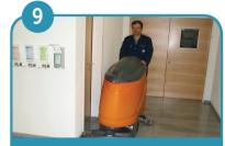
Clean the floor. When re-filling the tank and after use always switch off the machine with the key switch.
