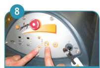
Start vacuum motor, start & adjust solution flow.
