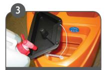
Dose cleaning product into dosing aid, pour it into the solution thank. Then rinse the dosing aid and close the solution tank with it.
