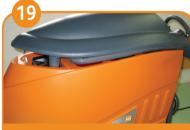
Store machine with partially open lid (lid rests on dosing aid) for ventilation.
