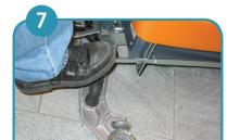
Lower the brush unit. The brushes should then couple to the unit automatically. If not repeat from pt. 5 on.
