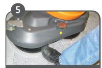
Position tool(s) precisely under the lifted brush unit.
