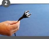
Check equipment, especially plug and cable. Report any fault or damage to a supervisor.
